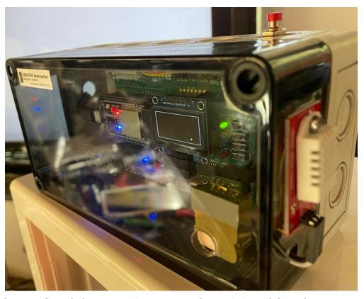
The data can be transferred via NBIoT, GSM, Lora, ModBus RS485, WiFi & Ethernet communication types. All HTTP and MQTT data streams are encrypted following the AES-256 CBC standard.
